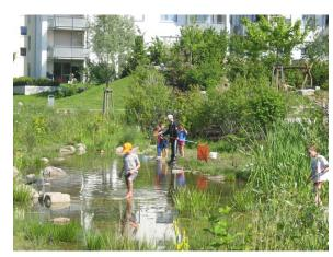
Shallow slopes, low water depth and stable edges minimise the need for fences and illustrate a designled approach to health and safety
